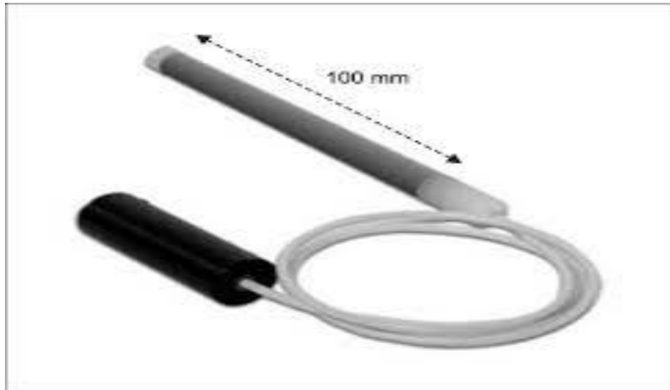
Figure 4 the Ionisation chamber (CC04)
